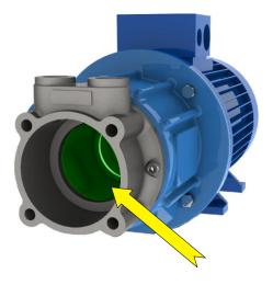
Before to insert the new cartridge, carefully inspections the internal of rear casing, to check the presence of damages, like signs of friction, signs of overheating or dents.
