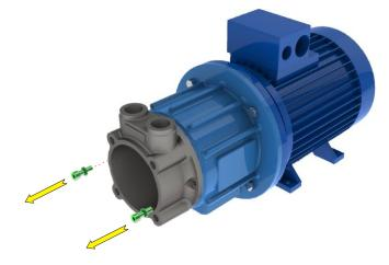
In case the rear casing is compromised, it is necessary to replace it.
