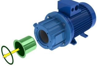
Now is possible to pull out the pump casing.
