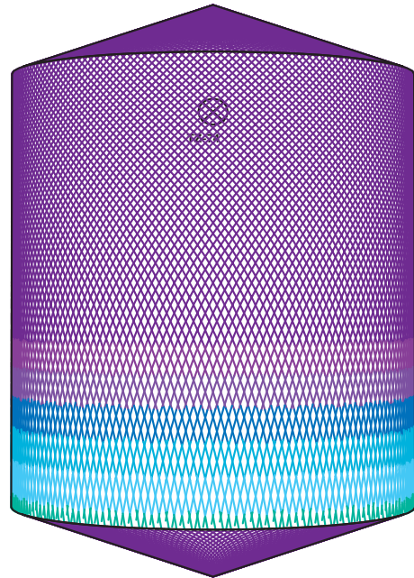
D5m H6m, Toftejorg TZ-74 Self Cleaning version, 4 x ø7 mm, 0% Time = 15.3 min., Water consumption = 4853 l
