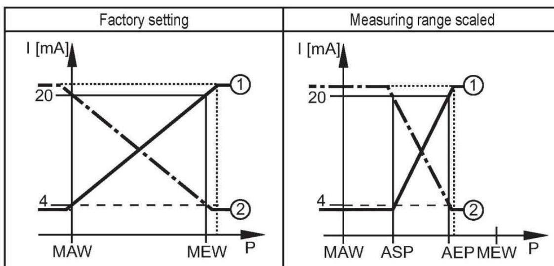
P = system pressure , MAW = initial value of the measuring range, MEW = final value of the measuring range
