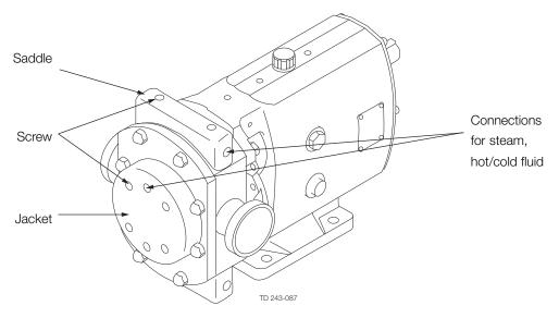
The maximum allowable pressure and temperature of heating/cooling fluid is 3.5 bar (50 psi) and  $150^{\circ}\text{C} (302^{\circ}\text{F})$  respectively, except in T4 applications in which the maximum allowable temperature is  $130^{\circ}\text{C}$ .
