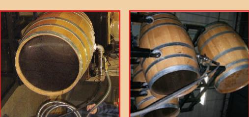
High performance 360° impingement cleaning scours the barrel interior, while an integrated vacuum extracts the liquid. The vacuum is powerful enough to extract the lees and gives you the option of using it to rack the wine.
